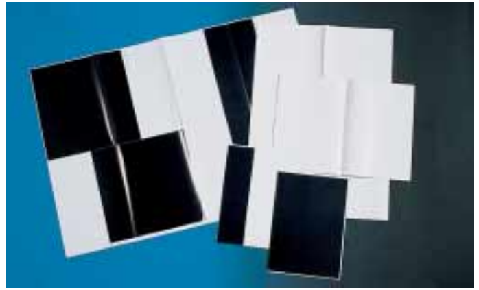
Fig. C Printed and unprinted sheets folded to 16 pages. In combination, the printed sheets simulate plates bled off in the binding.
